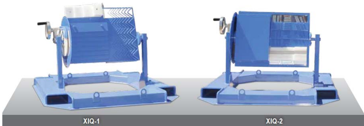
Figure 1. ANSTO image quality test objects.
